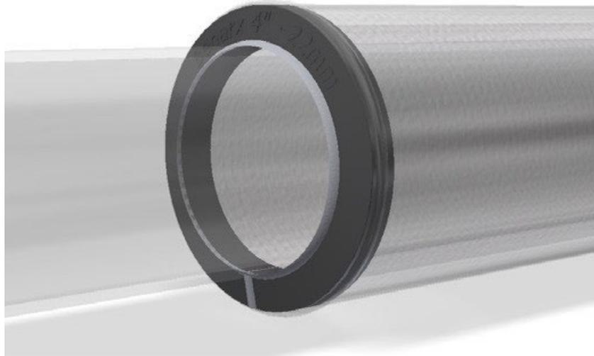
The end termination of pipe insulation is a critical point for prevention of water ingress into the pipe insulation material. The installation of metallic end caps may be challenging with respect to water ingress and can potentially damage the pipe coating due to sharp metal edges as a result. This leads to a major risk for development of CUI.
