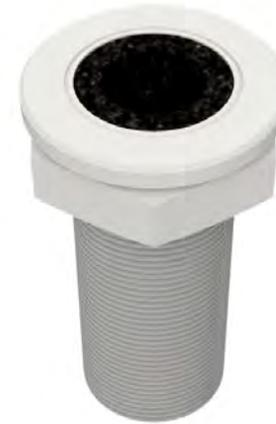
**Benarx® Fire Drain Plug is an effective and automatic drainage system. It functions as ventilation (air-flow) with dissipate heat/gas build-up away whilst maintaining fire integrity during the fire as it will seal off the hole by swelling.**
